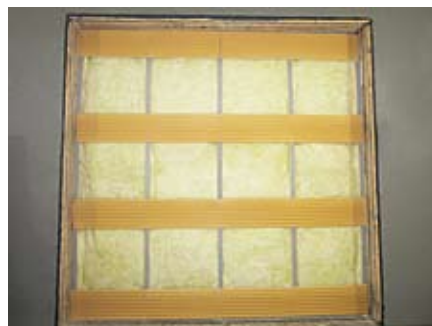
4 #1043 - Secondary Insulator, snapped on primary insulator
