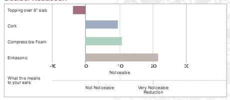
Note: Tests were performed with no ceiling assembly on 1' x 3' sample, marble thinset to a 4" slab.
